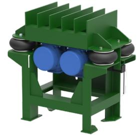
The empty box, carton or drum is rolled into position over the grid top which is in the lowered position. Upon starting, the grid deck is raised by inflating air mounts and the load is elevated off the roller conveyor surface. The contents are then compacted or settled inside the container. Upon completion of the vibrating cycle, the container is lowered back onto the conveyor and advanced to the next operation.
